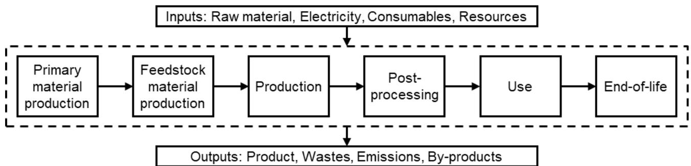
**Figure 1. Life cycle stages of an additively manufactured part.**
