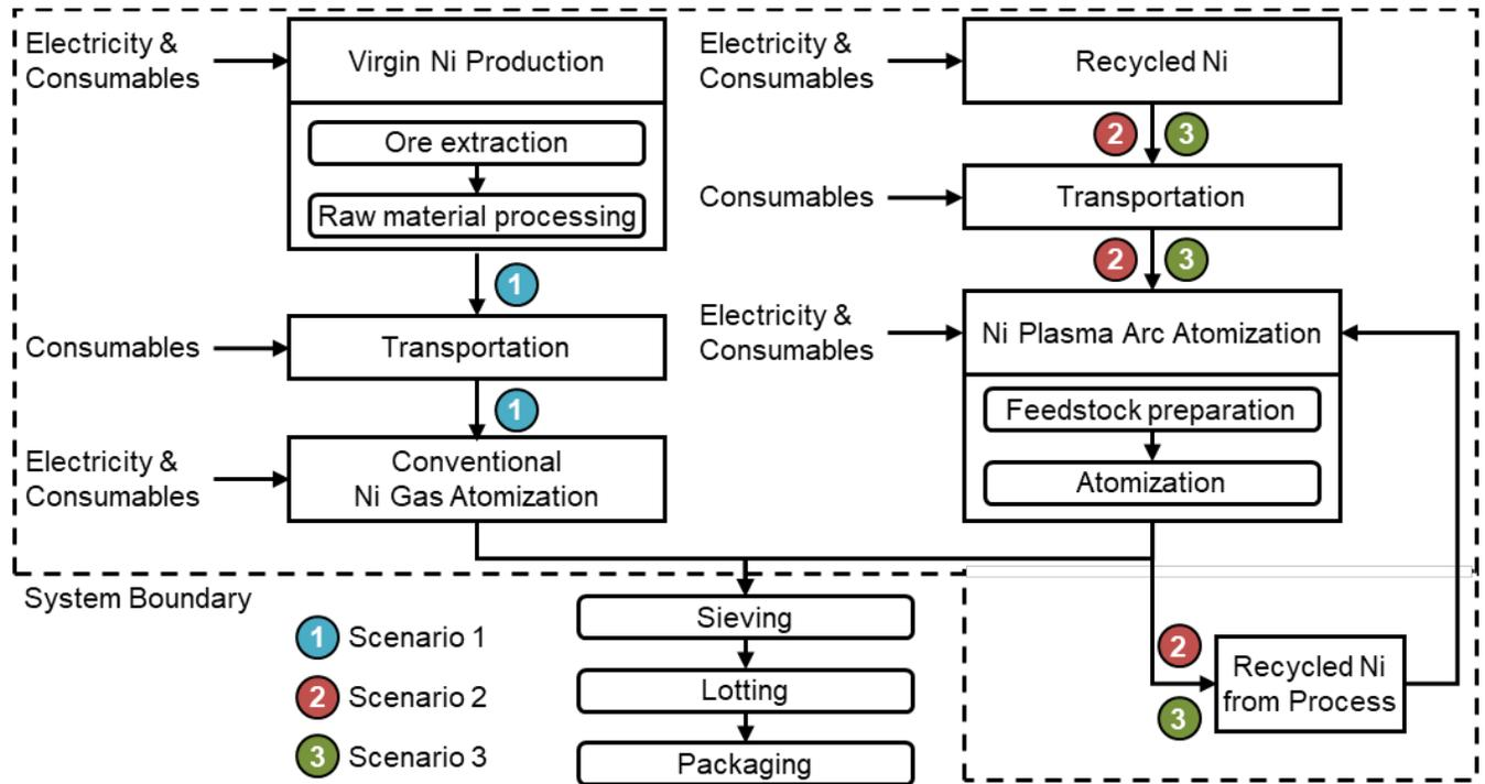
**Figure 3. Scenarios for making Ni powder using virgin and recycled raw materials.**
